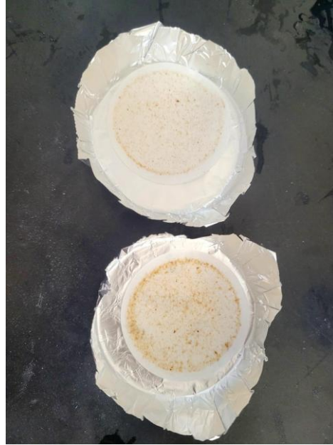
Figure 1. Total suspended solids. Top: suspended solids collected from the 250 mg L -1 treatment; bottom: suspended solids collected from the 350 mg L -1 treatment.
