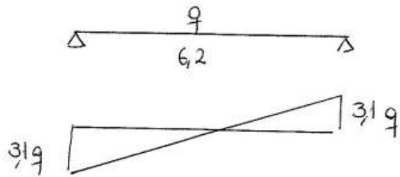
a)  $V_{max} = 31g \quad V_{dmax} = 4,34g \quad \alpha v = 0,9 \quad V_{rd2} = 529,39 \text{ kN}$
