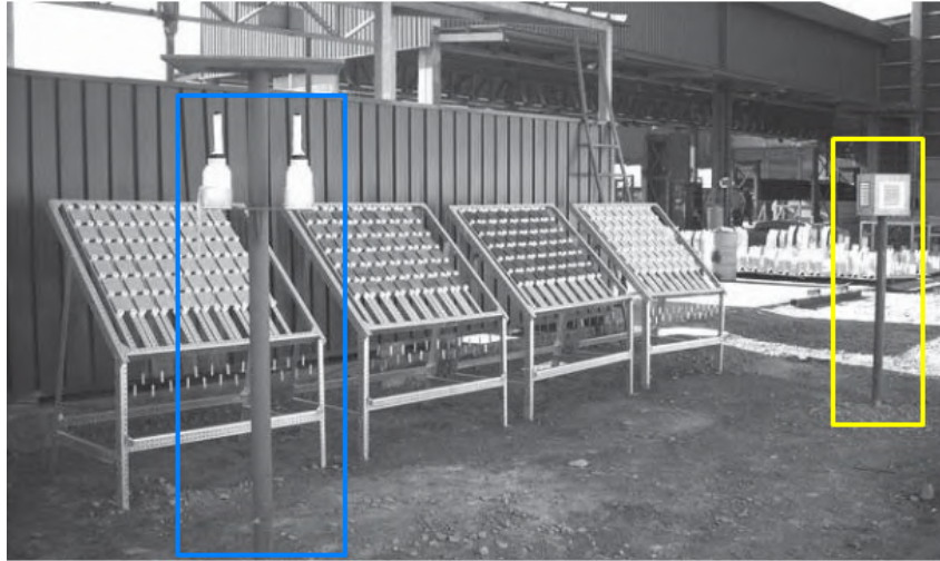
Figure 2 – Atmospheric corrosion station. The sample racks are in the center, with the candle for chloride ions highlighted by the blue box on the left and the candle for sulfur dioxide highlighted by the yellow box on the right.
