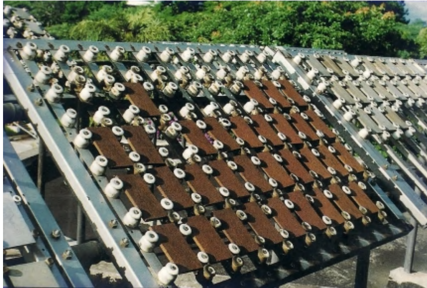
Figure 1 – Example of a rack that follows the methodology of international atmospheric corrosion standards.
