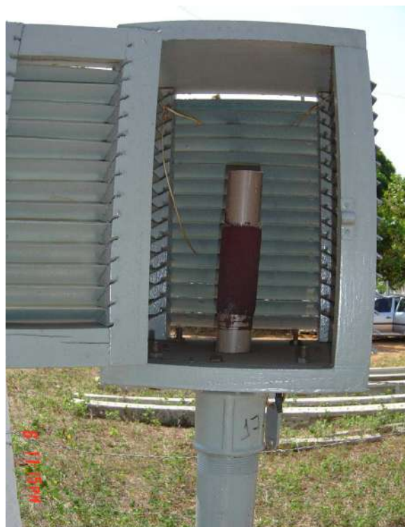
(b) A lead dioxide sulfation cylinder. Source: (GIRÃO, 2007)
