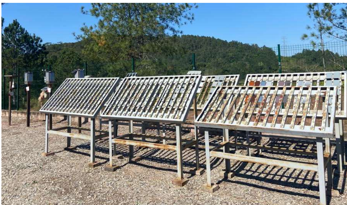
Figure 4 – An example of an atmospheric corrosion station: from left to right, one wet candle for chloride pollutants, three lead dioxide sulfation cylinders inside shelters, and six metal exposure racks.
