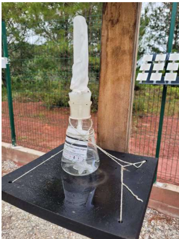
(a) An Chloride Wet Candle. Source: (BRANDENBURG, 2024)
