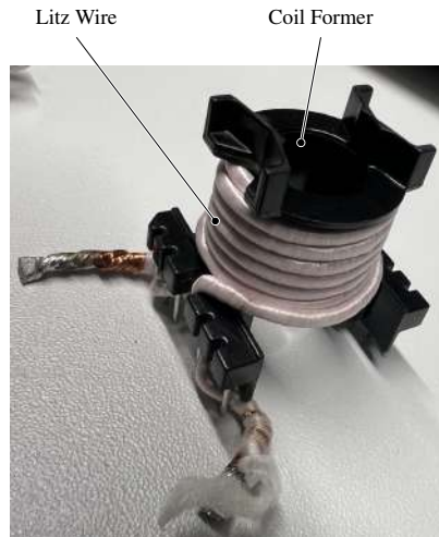
Figure 61 – Resonant Inductor Design and Built for the purpose of validating the proposed 4L-RFLCC.
