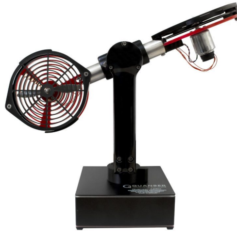
Figure 11 – Quanser AERO didactic plant.
