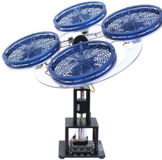
Figure 16 – Quanser 3DOF Hover didactic plant.
