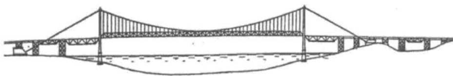
Figure 4. Schematic of a design (not adopted) for a suspension bridge at Florianopolis (Steinman 1929).
