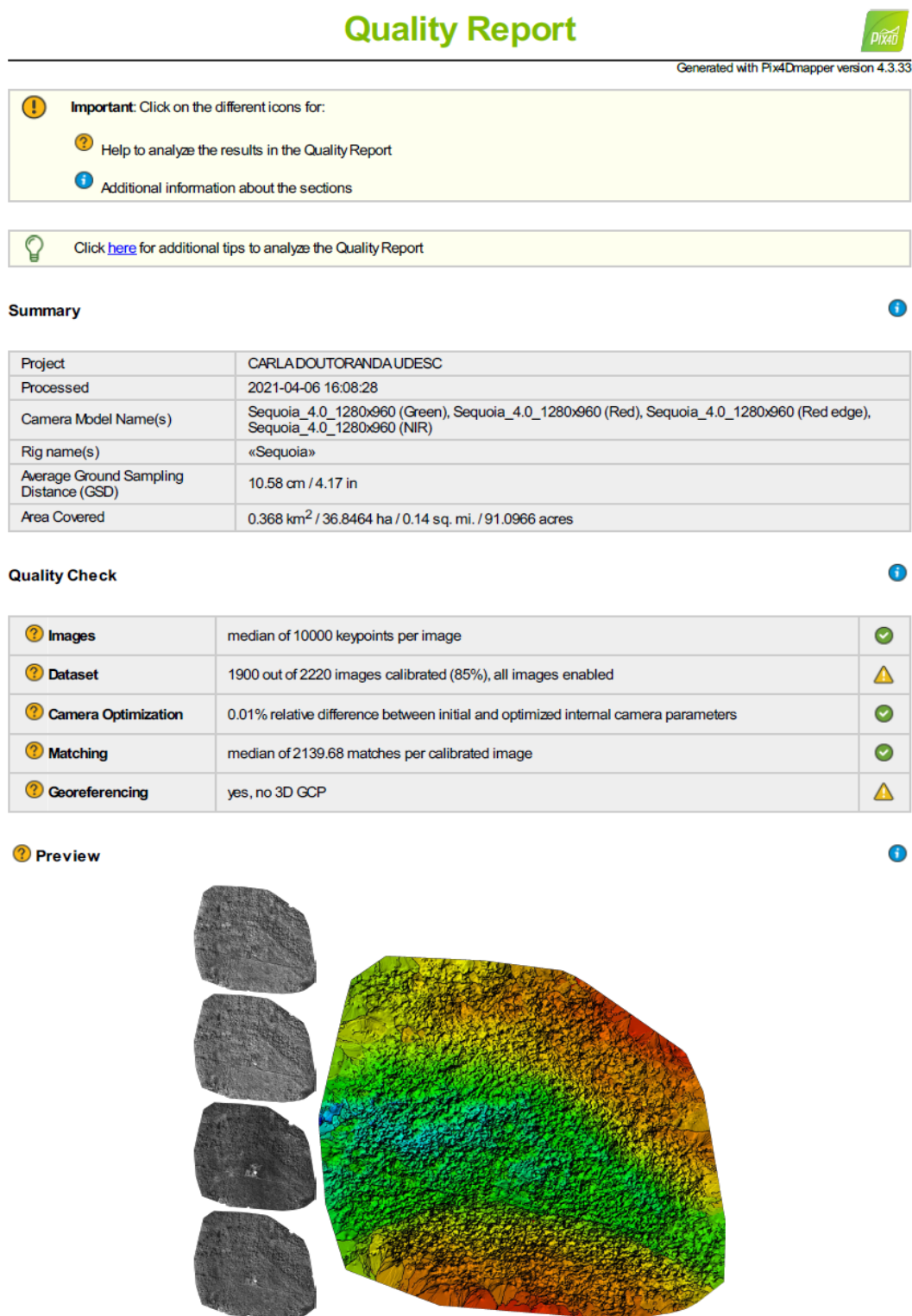
Figure 1: Orthomosaic and the corresponding sparse Digital Surface Model (DSM) before densification.
