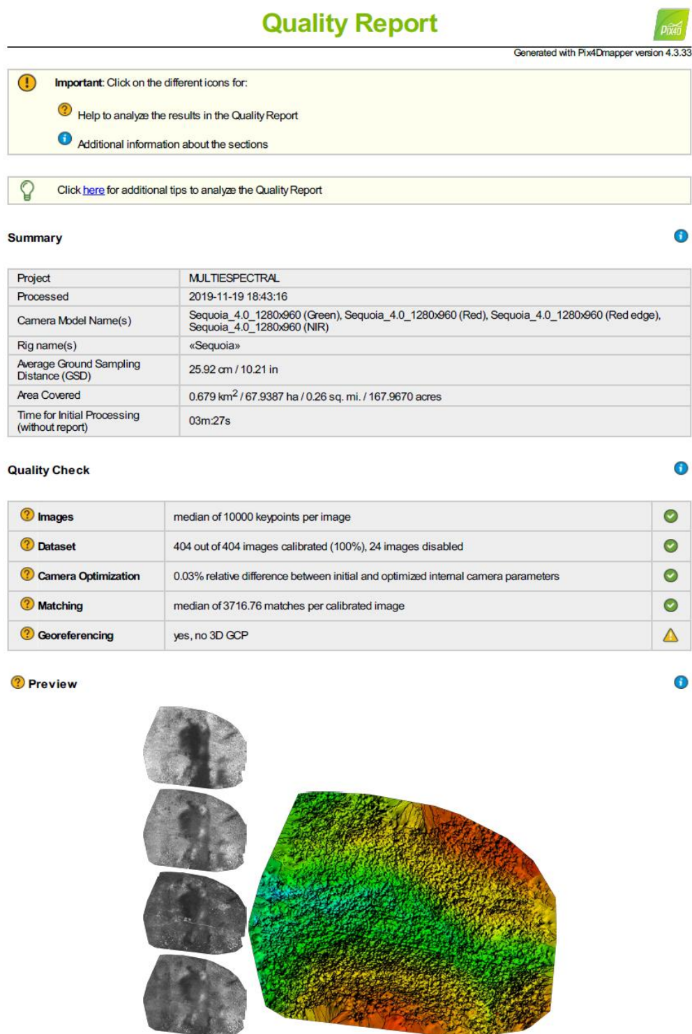
Figure 1: Orthomosaic and the corresponding sparse Digital Surface Model (DSM) before densification.
